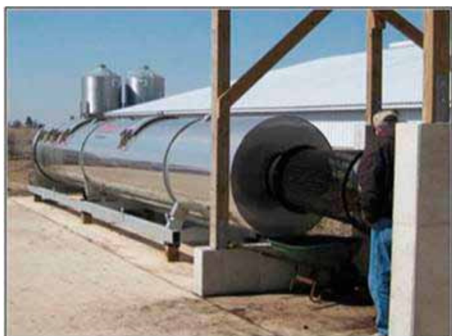
Figure 11 Biovator® discharge end with bone screen
