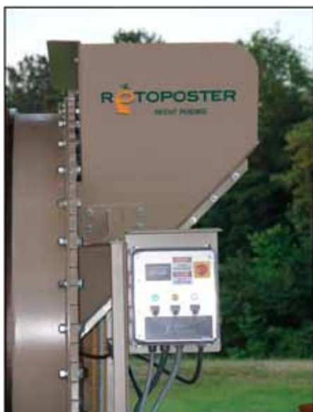
Figure 7 Rotoposter™ bone screen at discharge end
