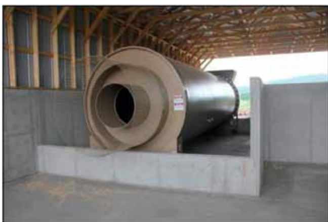
Figure 7 Rotoposter™ bone screen at discharge end
